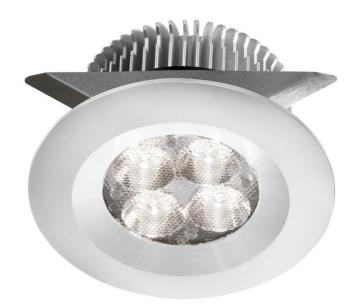
White 2x4W 3000K, CRI80+, 25° beam, 24VDC input with Male Connector, 18" Lead wire, D70xH50 mm, Dimmable.
