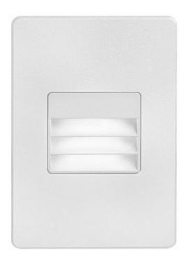
120VAC input, L125mmxW78mmxH37mm, 2700K, 3.3W IP65, White Wall LED Light with Louver
